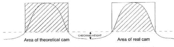
Cam Factor = 100 x (Area of real cam + Area of theoretical cam)
